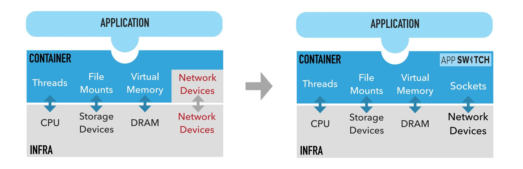
AppSwitch enables the container to work with an OS level abstraction for network and remove requirement for additional privilege
